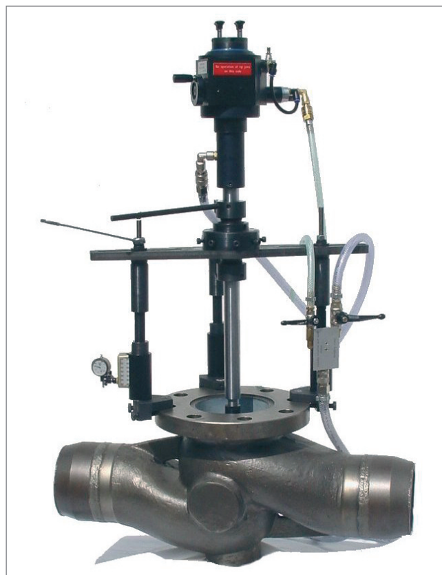
HTS 150 grinding sealing surface in 6" Control valve
