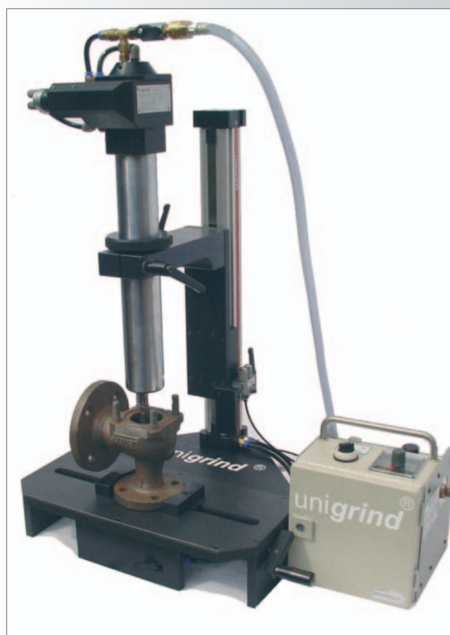
Grinding/lapping a Safety Relief Valve with SVS 1
