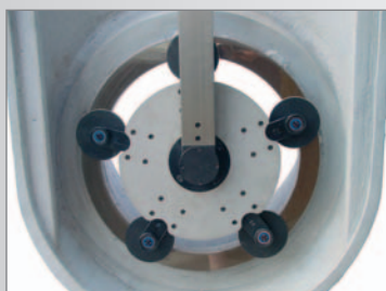
Planet disk with continuous adjustable grinding heads
