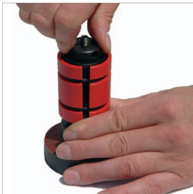
Grinding tools are guided and centred in the bore using adjustable expansion mandrels.
