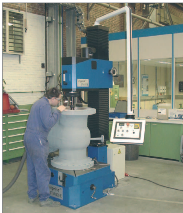
Grinding Gate Valve with STM 800 E
