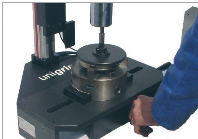
Grinding/lapping a valve disk with SVS 1 on machine stand
