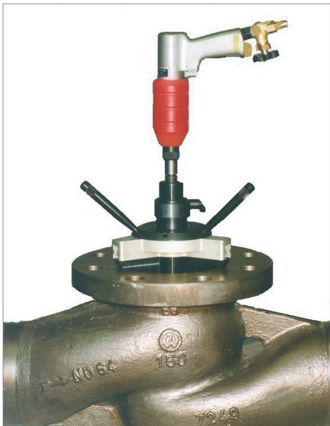
KVS machine with 3-jaw chuck mounted on 6" control valve
