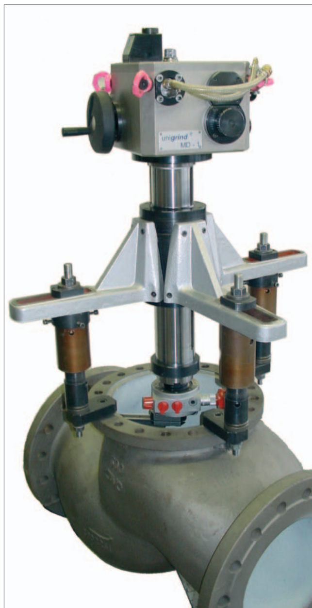
MD 1 machining globe valve seat
