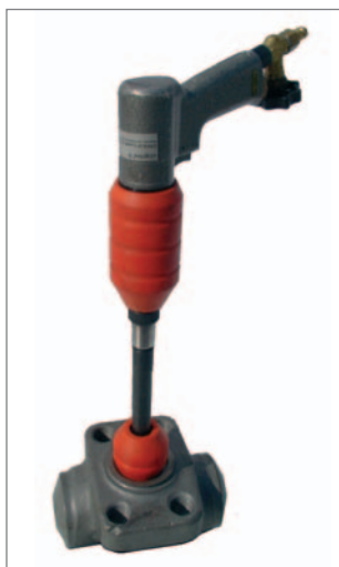
KVS machine grinding 1" globe valve
