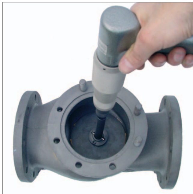
Grinding the valve seat with VENTA 150
