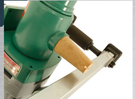
Sound absorber (sintered metal) - turnable -
